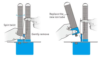
1.Gently move away the power sheet metal.Pinch the ion tube counterclockwise twist for a few turns, you can take it out.
