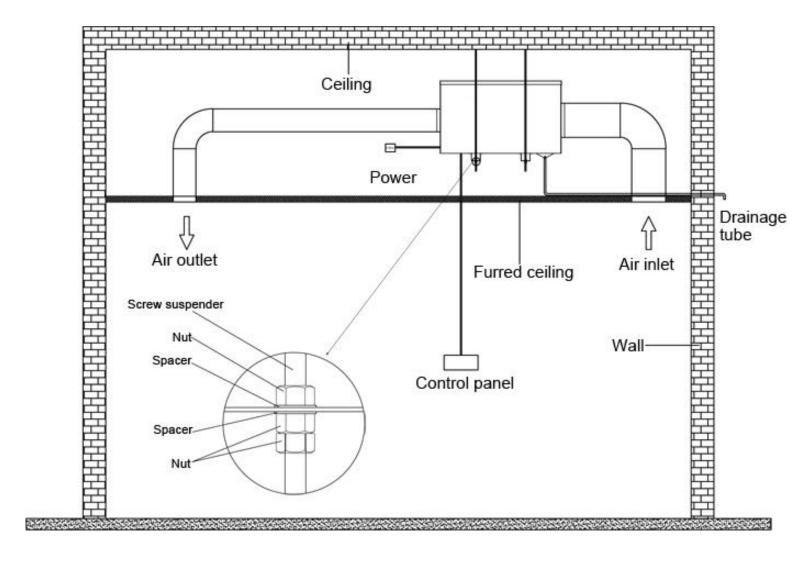
Attention: Install the machine stably with screw suspender on the ceiling, and make sure installation in flat.
